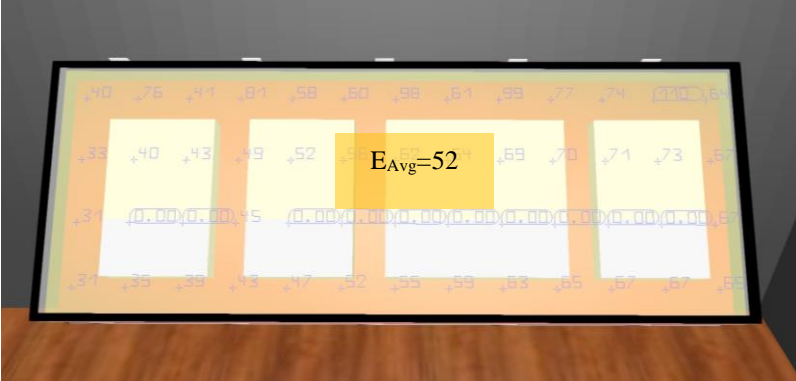
Figure 4.32. Light level calculation results (in lux) for highly susceptible books in Room 2
