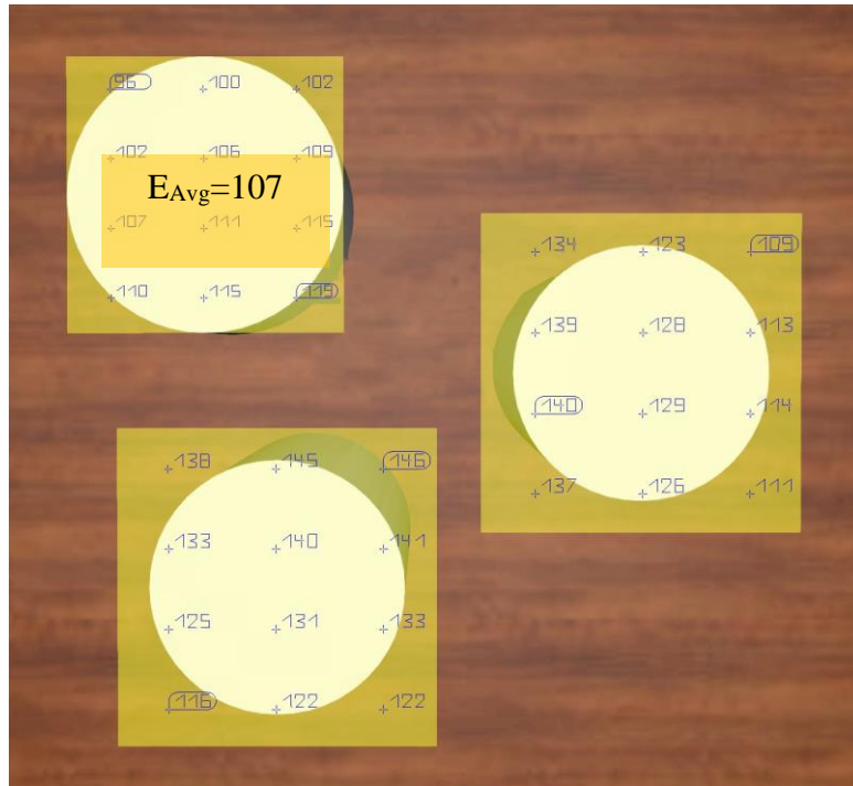
Figure 4.25. Light level calculation results (in lux) for moderately susceptible luggage on platforms in Room 1
