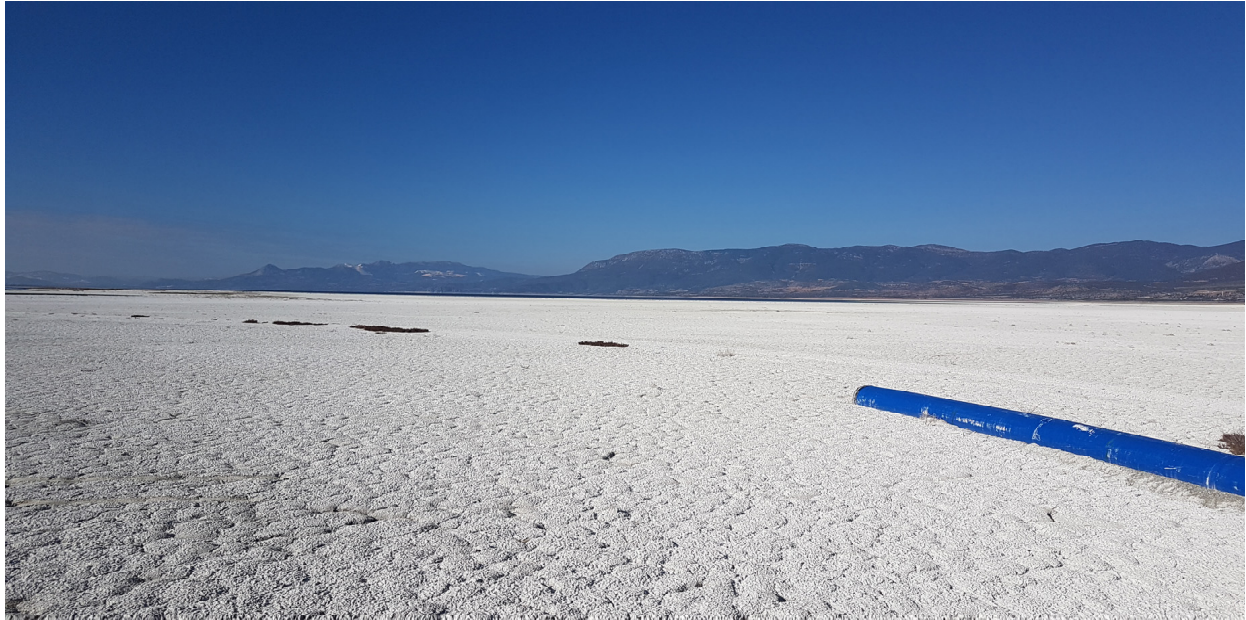
Figure 1. The ruptured pipeline on the Burdur Lakebed was exposed due to the lake's drying.
