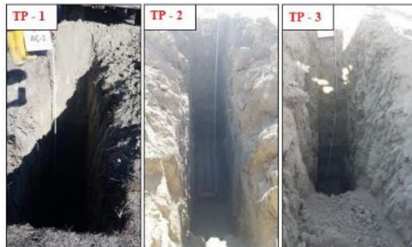
Figure 22. Three of the seven exploratory trial pits were excavated at the site.
