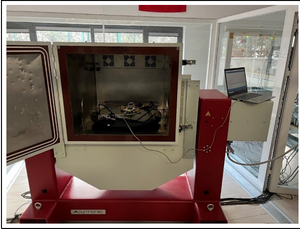
Figure 1. Measurement test setup for Pololu IMU01b.
