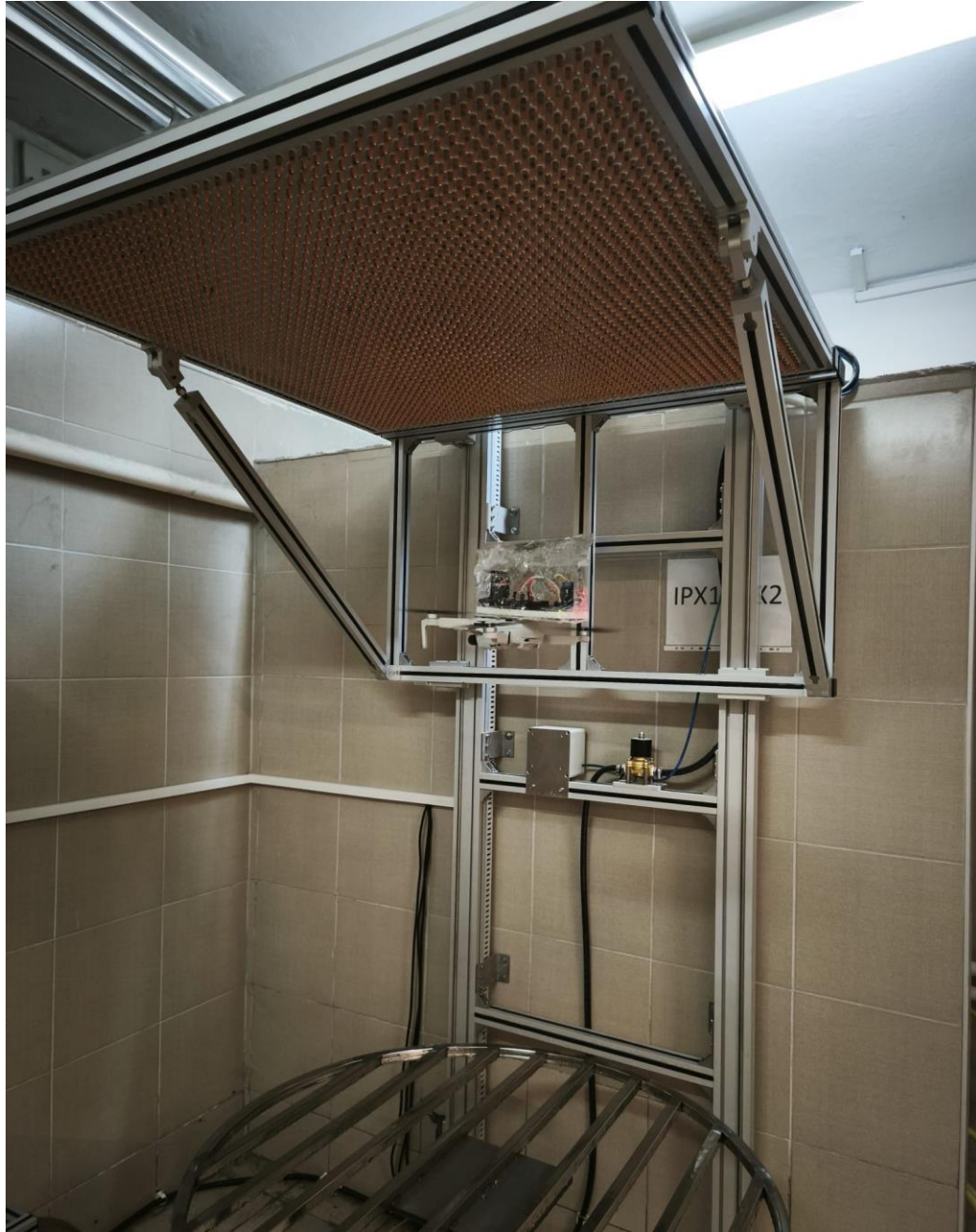
Figure 3.19. Indoor IPX2-Compliant Rainfall Simulation Setup Used for Testing the IMU Performance under Controlled Water Exposure
