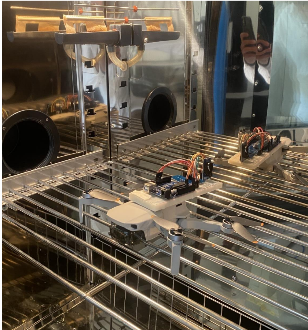
Figure 3.14. UAV and Externally Mounted MPU6050 IMU Module during Pre-Conditioning Phase Inside the Environmental Test Chamber
