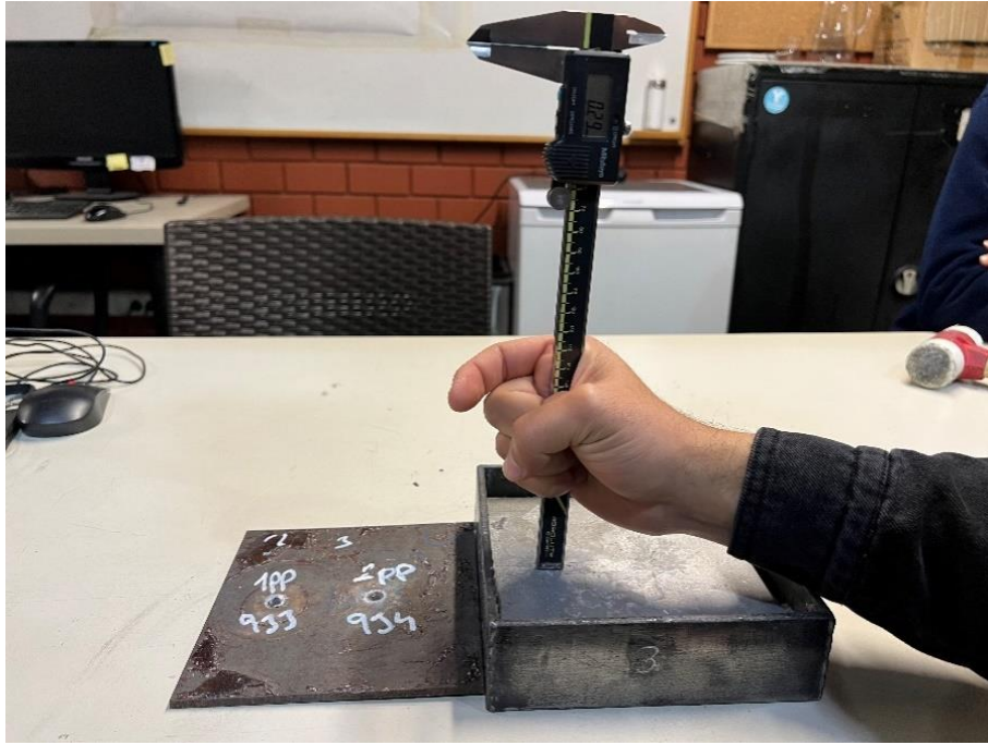
Figure 4.34. Depth of Penetration on Backing Plate After First Impact of Configuration – 5 (0,29 mm)
