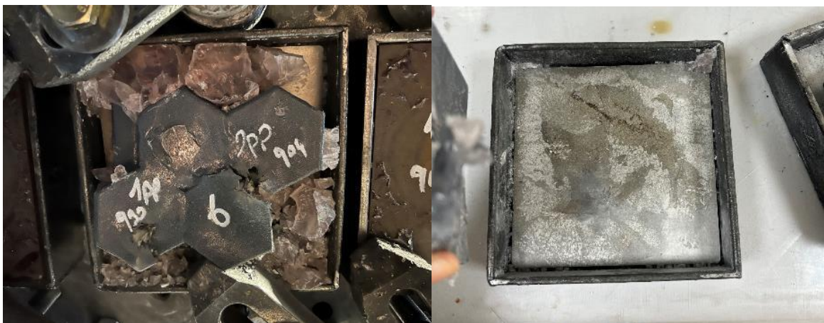
Figure 4.31. Detailed Visuals of Configuration – 4 after Ballistic Impact (Impact Velocities: 930 m/s and 904 m/s)
