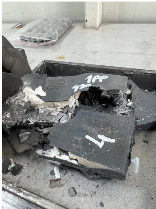
Figure 4.38. Broken Ceramic Tiles of Configuration – 6 after Ballistic Impact
