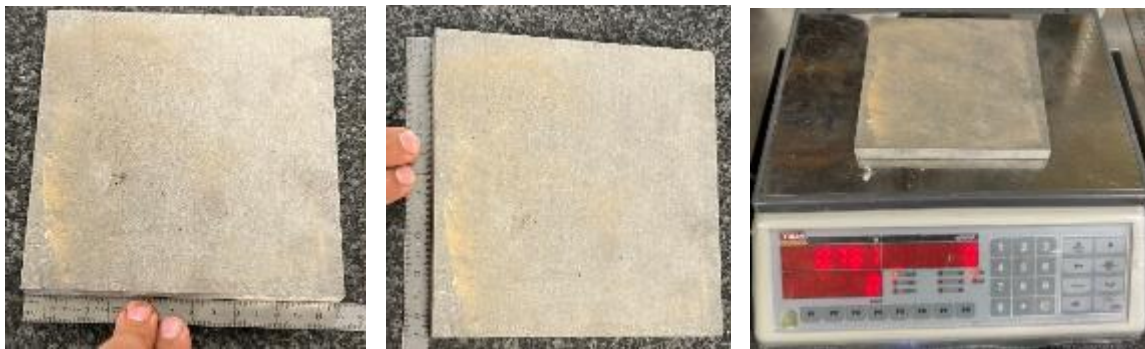
Figure 4.17. Dimensions and Mass of the Aluminum Backing Layer
