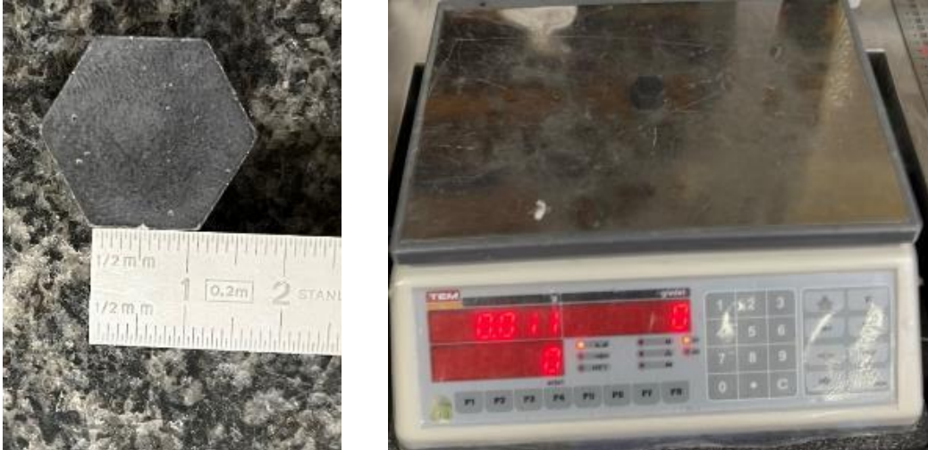
Figure 4.15. Dimensions and Mass of the 10 mm x 10 mm SiC Hexagon Tiles
