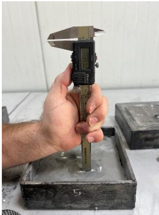
Figure 4.24. Depth of Penetration on Backing Plate After First Impact of Trial Configuration – 2 (1,93 mm)
