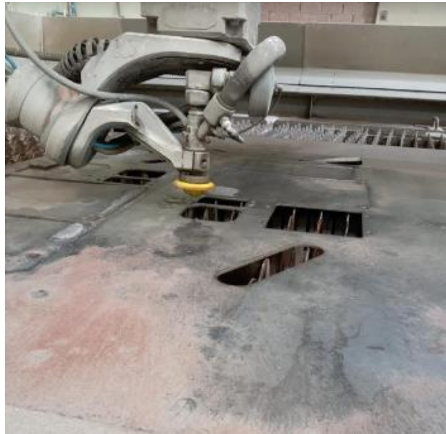
Figure 4.8. Steel Cutting Process with Waterjet
