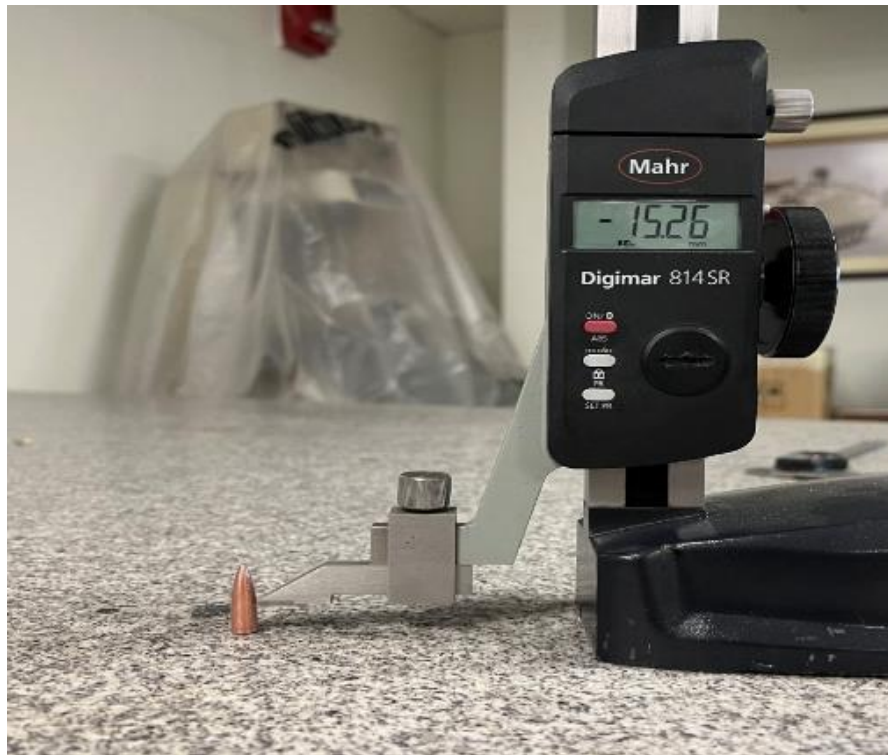
Figure 5.1. Measurement of Nose Length of the Projectile
