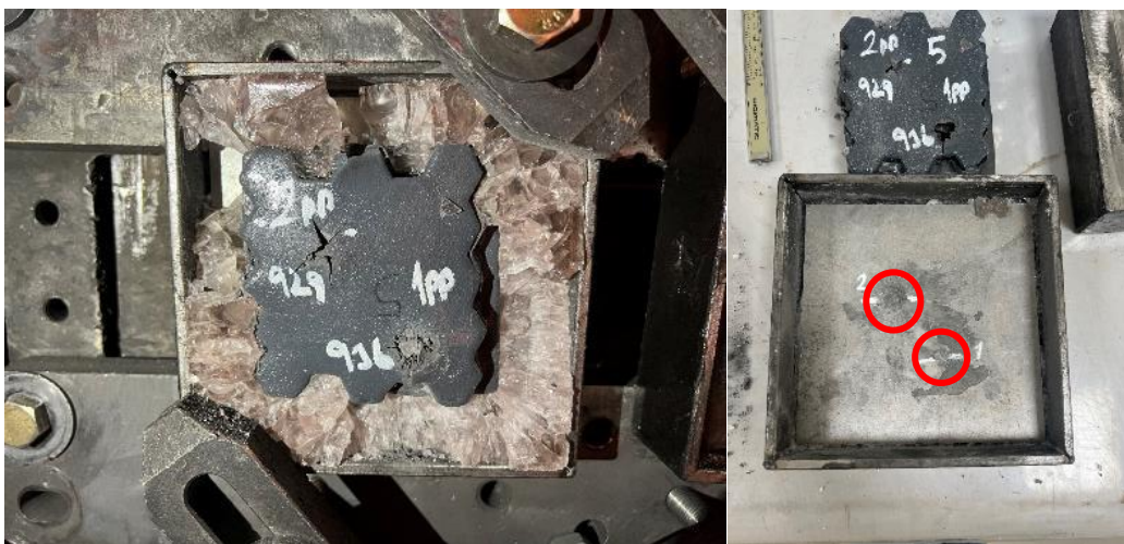
Figure 4.23. Detailed Visuals of Trial Configuration – 2 after Ballistic Impact (Impact Velocities: 936 m/s and 929 m/s)
