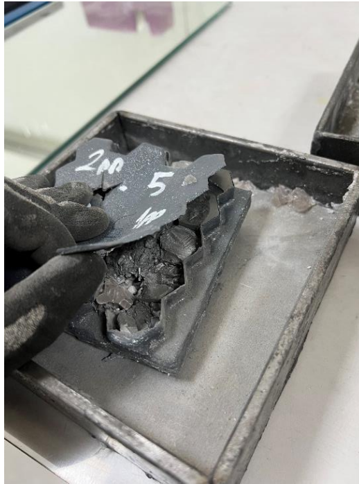
Figure 4.26. Broken Ceramic Tiles of Trial Configuration – 2 after Ballistic Impact
