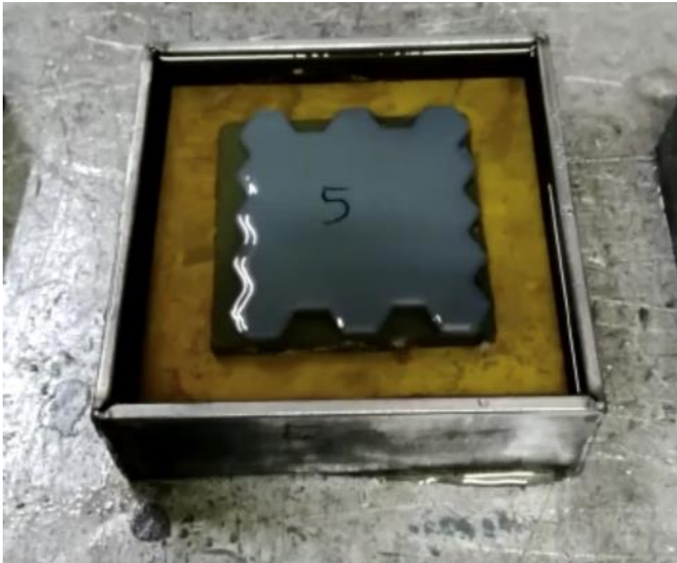
Figure 4.12. Epoxy Resin Application to Ceramic Tiles
