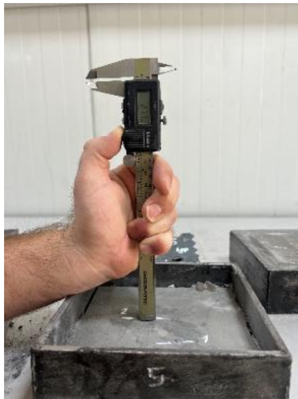
Figure 4.25. Depth of Penetration on Backing Plate After Second Impact of Trial Configuration – 2 (2,77 mm)
