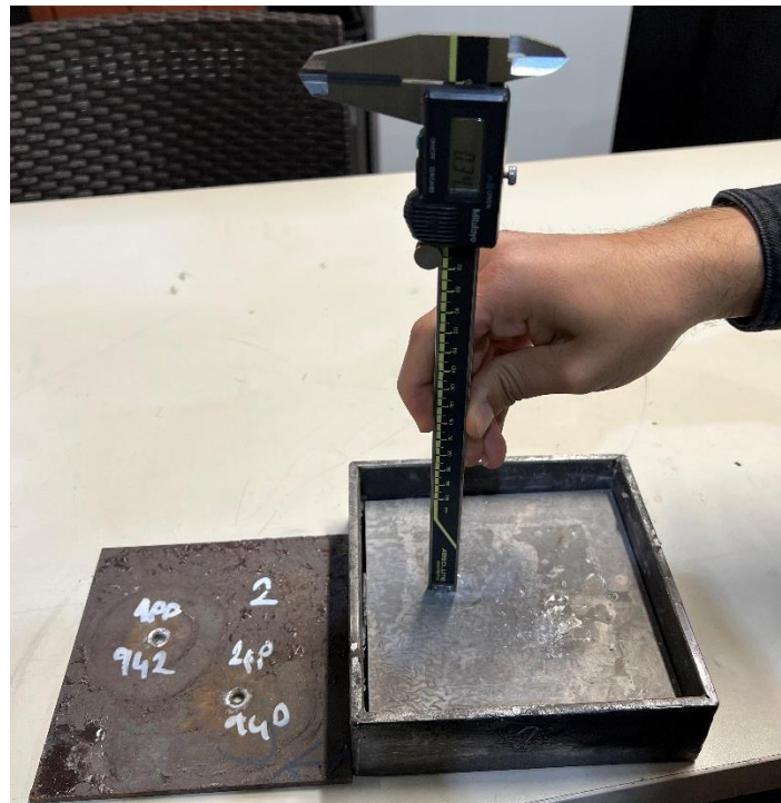
Figure 4.21. Depth of Penetration on Backing Plate After First Impact of Trial Configuration – 1 (0,34 mm)
