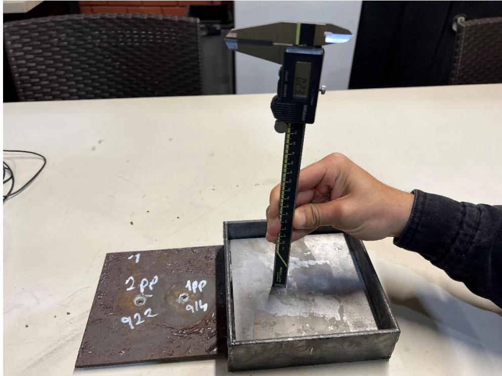
Figure 4.30. Depth of Penetration on Backing Plate After Second Impact of Configuration – 3 (0,23 mm)
