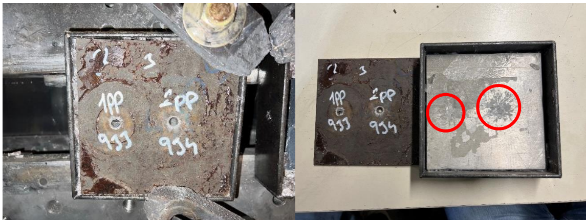
Figure 4.33. Detailed Visuals of Configuration – 5 after Ballistic Impact (Impact Velocities: 933 m/s and 934 m/s)
