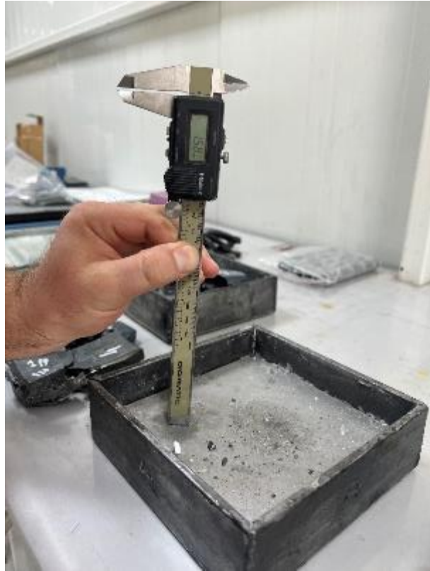
Figure 4.37. Depth of Penetration on Backing Plate After Second Impact of Configuration – 6 (1,58 mm)
