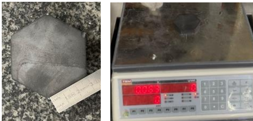
Figure 4.14. Dimensions and Mass of the 30 mm x 30 mm SiC Hexagon Tiles
