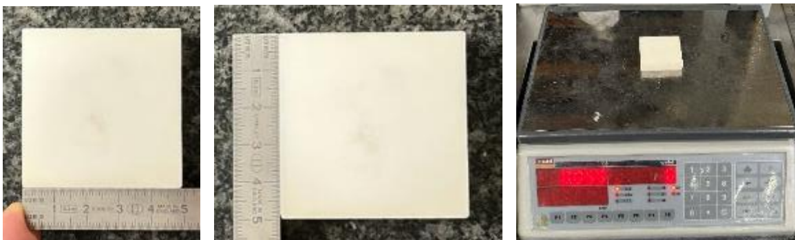
Figure 4.16. Dimensions and Mass of the Alumina Tiles
