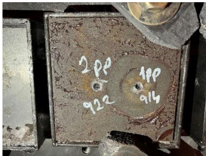
Figure 4.27. Front Plate Visual of Configuration – 3 after Shootings (Impact Velocities: 914 m/s and 922 m/s)
