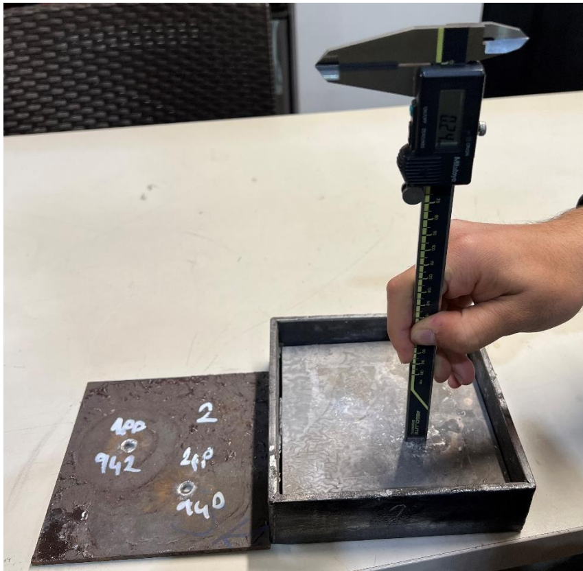
Figure 4.22. Depth of Penetration on Backing Plate After Second Impact of Trial Configuration – 1 (0,24 mm)
