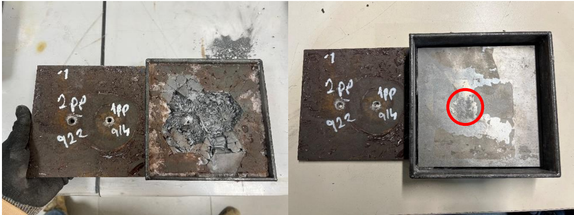
Figure 4.28. Detailed Visual of Configuration – 3 after Ballistic Impact (Front Layer, Ceramic Core – 1 & Back Plate)
