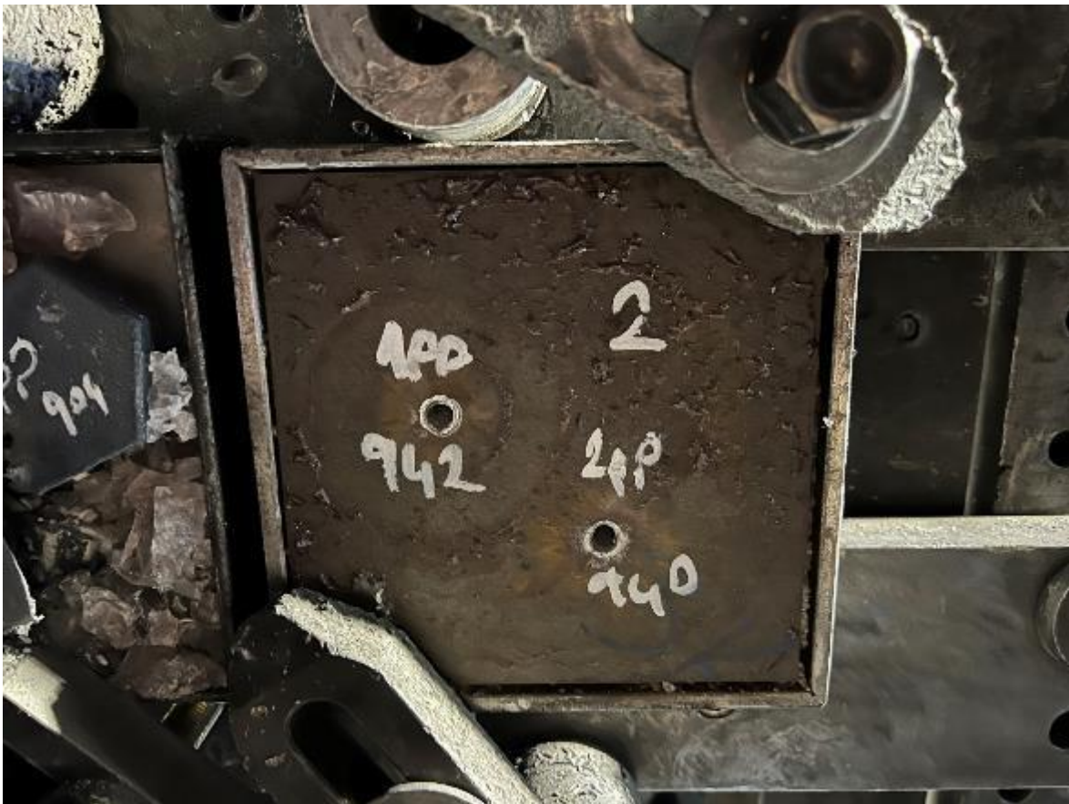
Figure 4.19. Front Plate Visual of Configuration – 1 after Shootings (Impact Velocities: 942 m/s and 940 m/s)
