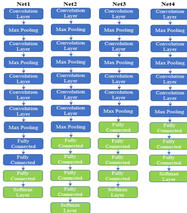
Figure 4.3. The graphical pipeline of the proposed CNN models. The transferred layers are shown in blue and green ones are newly added layers.
