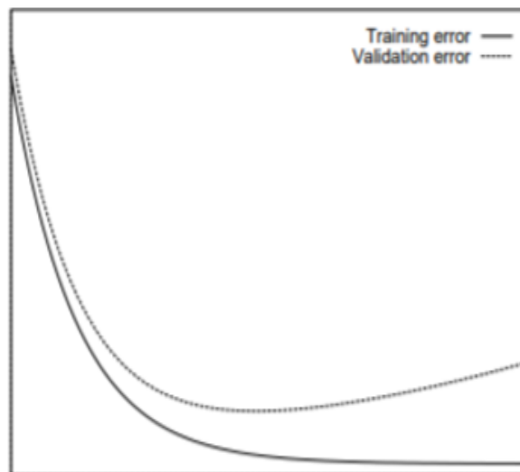
Figure 3.1. Idealized training and validation error curves. Vertical: errors; horizontal: time [43].
