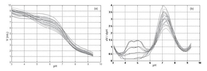
Figure 1. a) V vs. pH titration curves and b) dV/dpH vs. pH curves of selected training set solutions.
