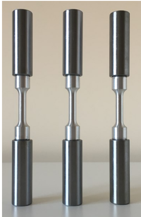
Figure 3.4 Test specimens of road wheel with steel assembly adapters
