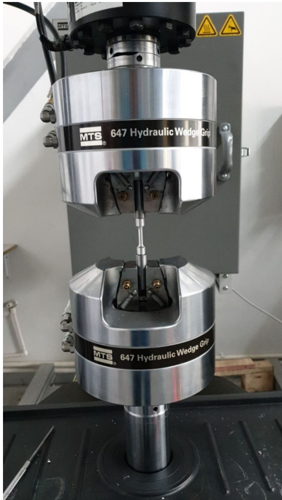
Figure 3.6 Fatigue testing of road wheel test specimens
