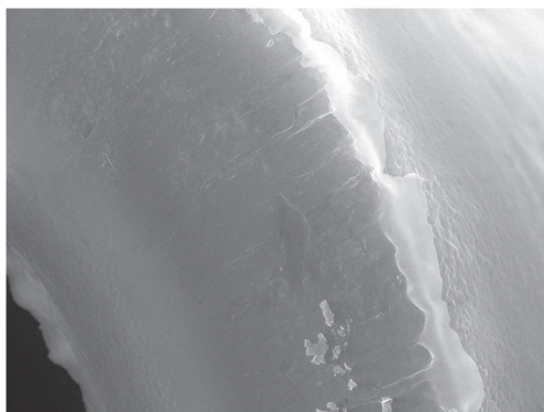
Fig. 2. Electron microscopic view of an uncoated oxygenator fibre.
