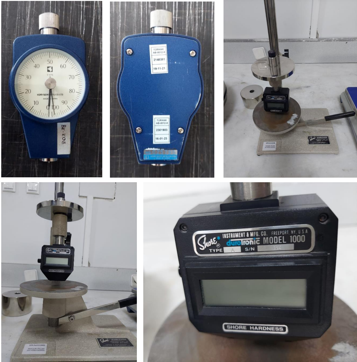
Figure 5.30. Shore Test Devices (Kori Durometer & Shore Leverloader).
