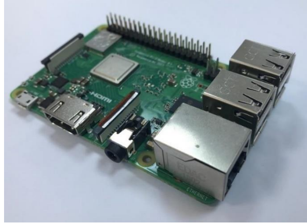
Şekil 3.1 Raspberry Pi 3 Model B+
