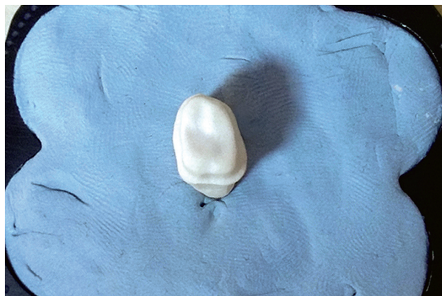
Figure 3. CAD-CAM–fabricated real-size cast of prepared tooth made of PU by using STL image of CBCT-scanned tooth without acrylic resin base (polyurethane cast fixed with silicone impression material before 3D laboratory scanning). CBCT, cone beam computed tomography; CAD-CAM, computer-aided design and computer-aided manufacturing.
