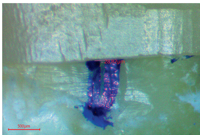
Figure 6. Vertical marginal discrepancy measurement (original magnification \times 100 ).
