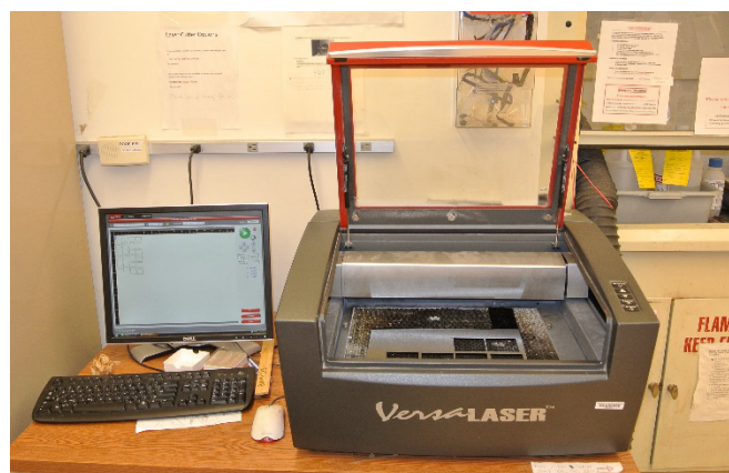
Figure 6.21 Laser cutter used in that thesis work. VLS2.3, Universal Laser Systems Inc.
