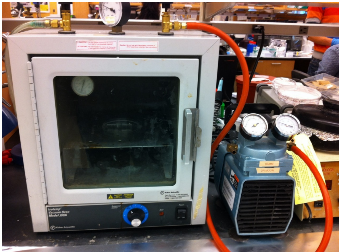
Figure 7.5 The vacuum oven for drying of chips, vacuum pressure is set to 600 mmHg and temperature is set to 37°C.
