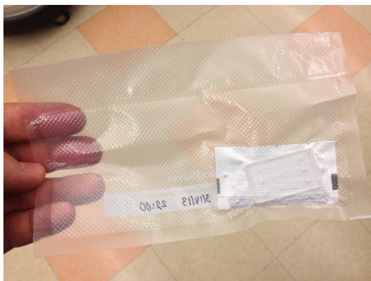
Figure 7.9 A functionalized chip, vacuum sealed with a bag of drying agent, ready for storing.
