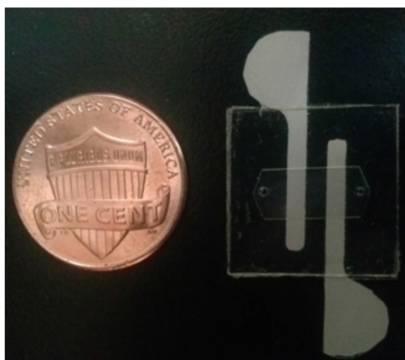
Figure 1.9 An example of a printed flexible plastic microchip. Silver electrodes are patterned using screen printing and channel is formed using a double sided adhesive (DSA) tape. [49]
