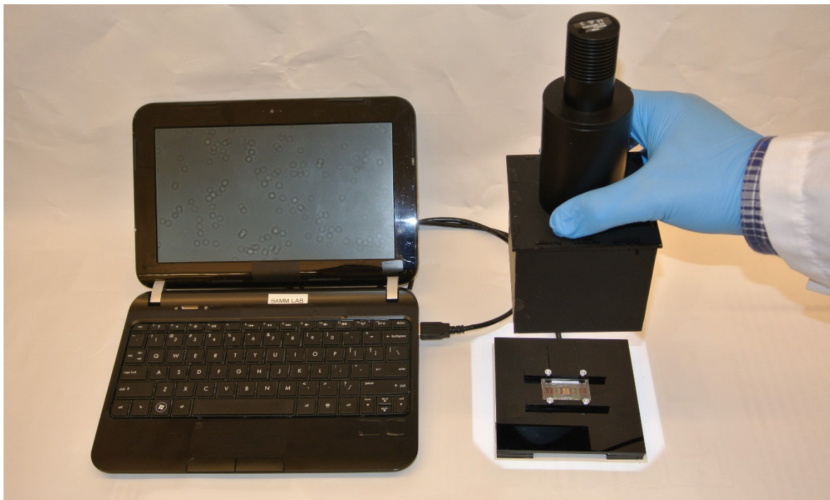
Figure 6.23 lensless wide-field microscopy system.
